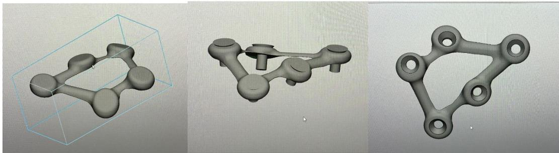
*Figure 14. Designing a plate. a) Place screw points and link them with bars. b) Add in screws in decide direction c) subtract screws to create hole.*
